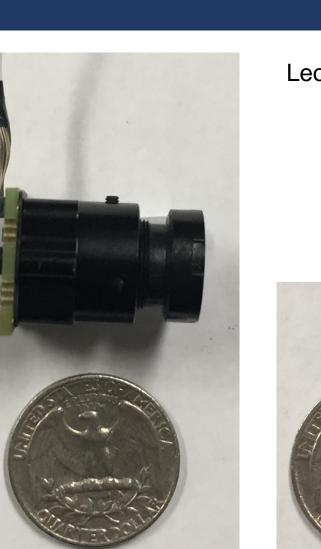
Leopard Imaging stereoscopic cameras (model number LI-OV580-STEREO).
